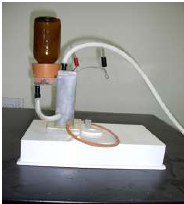
An electrolyser for the production of Chlorine, Hydrogen and Sodium Hydroxide from Brine
